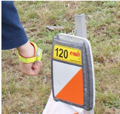
The "Proximity Reader" in action
